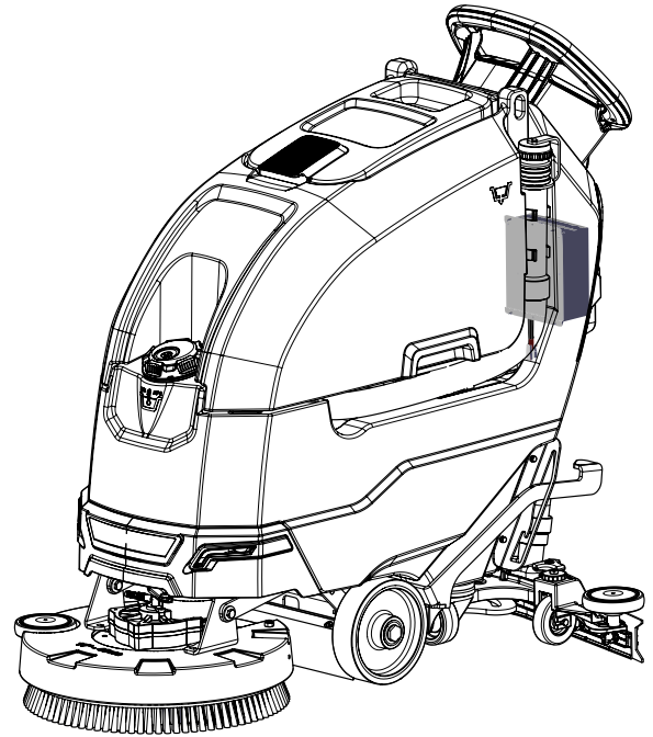
6 - ON-BOARD BATTERY CHARGER
